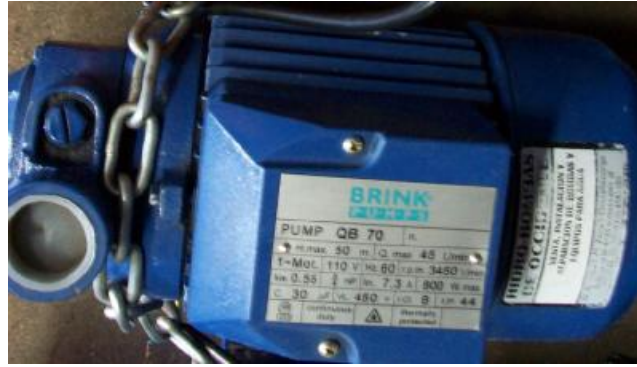
Figure 7.12 The Clarke TAM105 electric water pump [46] Figure 7.13 Sample photograph of the centrifugal water pumps available locally in Guatemala ( H_{max}=50m ; Q_{max}=45 l/min; P_{max}=800W )
