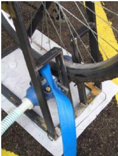
Figure 9.3 Photograph showing the outlet hose constriction
