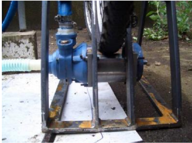
Figure 9.2 Photograph showing the clearance around the tyre
