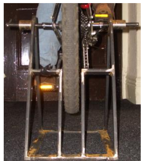
Figure 9.1 Photograph showing the negligible deflection of the axle grips when under full loading
