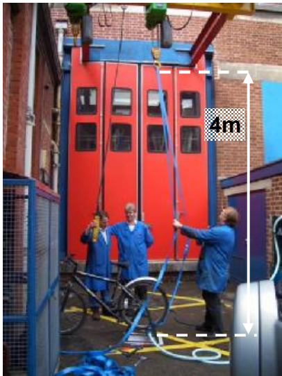
Figure 9.7 Winching up the hose to test the pump with a 4m head
