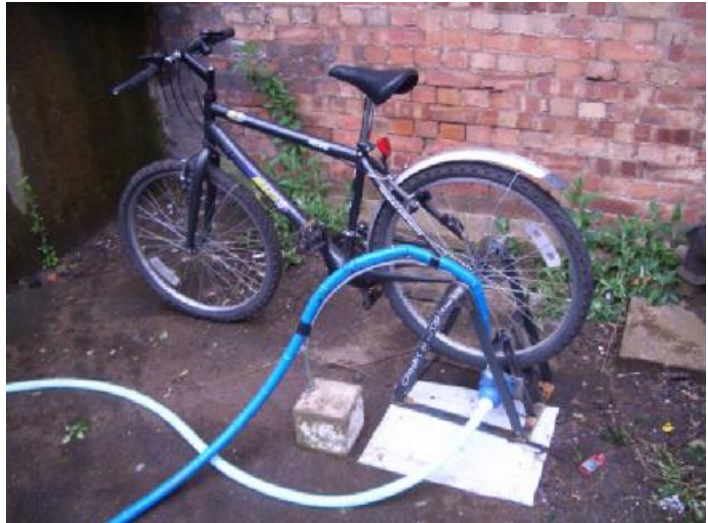
Figure 9.4 Photograph showing the modification to the outlet hose
