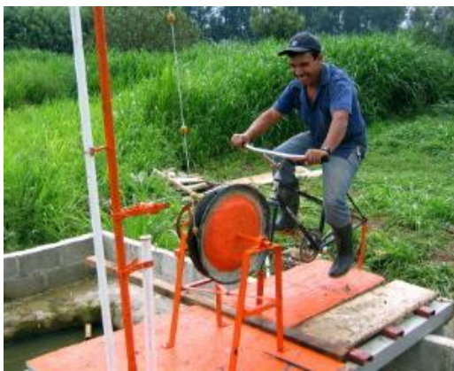
The Bicycle-Powered Well Pump
