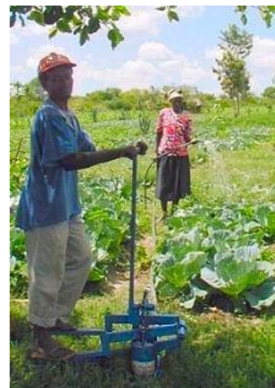
Figure 5.1 The MoneyMaker treadle pump [53]
