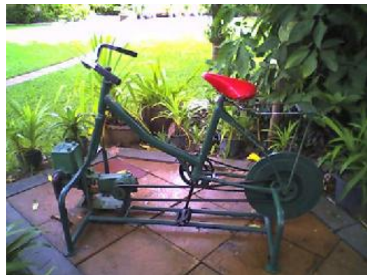
Figure 7.2 Bicycle powered water pump for watering the garden at C&C Hotel in Pattaya, Thailand [36]
