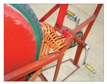
The outlet chute is made by spiraling remer bar around a metal tube. The shelled nuts spill out from here.
