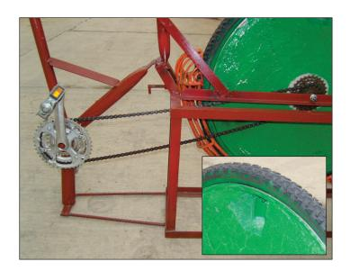
The flywheel is made by pouring concrete into a handmade mold. Mix 1 part cement with 2 parts fine sand. Make sure the valve is left uncovered for access and removal (see inset).
