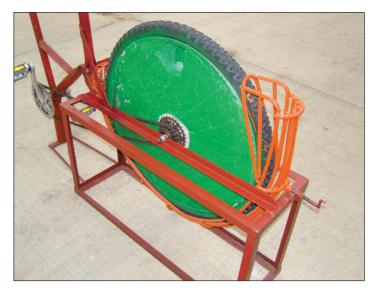
The chute is the most difficult part to make. It is made from remer bar, bent into shape around a bike wheel.
