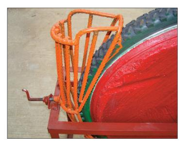
The entrance of the chute. The diameter of the chute is adjustable to allow for different sizes of nuts.
